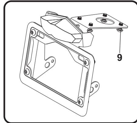
5. Route combination light wire through the hole in bracket and under passenger seat. Using the *BN-SSS-22-18* solder shrink connectors provided in the kit, connect the Yoshimura combination light wires to the stock brake light wires as follows:
